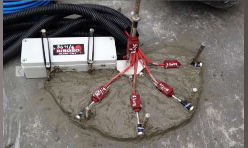
A Rosette of Embedment Strain Gauges
